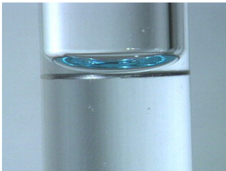
Figure: Meniscus over a measuring line.
